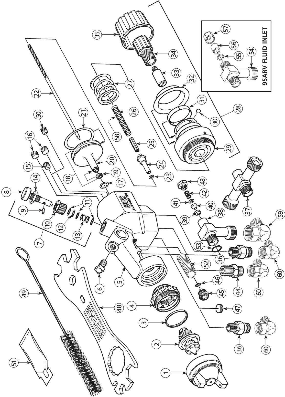
▲ Items (36) and (50) are for installations requiring separate fan and atomizing air control. Items are packaged loose. (See pg. 5)
