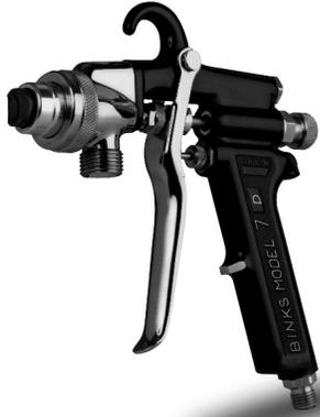
Designed for continuous spraying of heavy bodied fluids. Drop-forged aluminum body. Replaceable plated drop-forged brass head. Adjustable floating fluid needle valve. Stainless steel air valve cartridge. Trigger has hardened steel wear plate.
