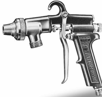
Designed for spraying heavy bodied fluids such as roof coatings, block fillers, and similar materials. Drop-forged aluminum body. Extra large fluid passage in plated drop-forged brass head. Adjustable floating needle valve and stainless steel air valve cartridge. Hardened steel four finger trigger. Controls at back of the spray gun. Non-adjustable spray pattern.
