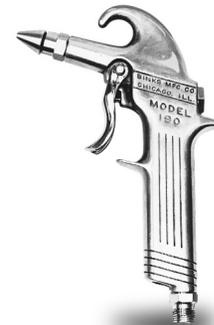
Use for dusting, drying, removing chips, etc. Pistol grip style with aluminum die cast body. Nozzle number 60-40 (complies with paragraph 50-204 Walsh-Healy Alt and OSHA where air inlet does not exceed 100 PSI) with 1/16" orifice is standard. Also available with 60-41 5-1/2" extension. 1/4" NPT (m) air inlet. Air consumption 3-1/2 CFM at 50 PSI. Part Sheet 77-1108
