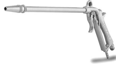
Use for spraying solvents to clean engines and other machinery. Brass body. Ten inch nozzle/tube length. Has flexible tubing with hose clamp for siphoning solvent from container. Requires 14 CFM air at 50 PSI. 1/4" NPS (m) air inlet. Part Sheet 77-1191
